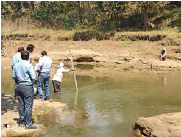
Figure 4 Onsite measurement of depth of flow and flow velocity of river
