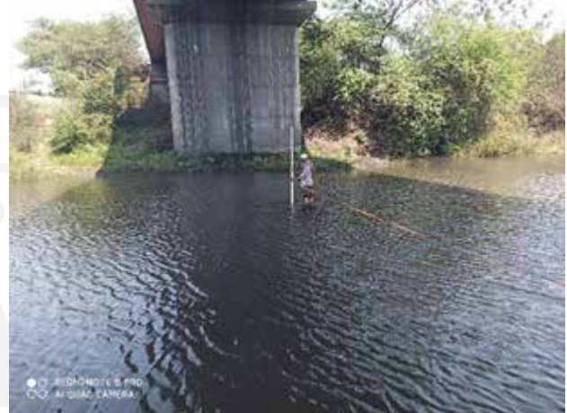
Figure 4 Onsite measurement of depth of flow and flow velocity of river
